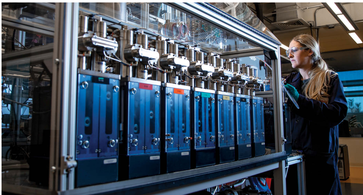
An ExxonMobil scientist works on a recombination cell used to combine gases with liquid oil at high pressure to produce a live oil mixture of fluid at in-situ reservoir conditions in support of calibrating advanced reservoir models.
