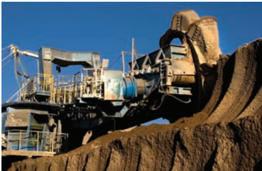
Stacker/reclaimer in action at the Mantoverde mine, which produced over 60 kt of copper cathode in the year.
