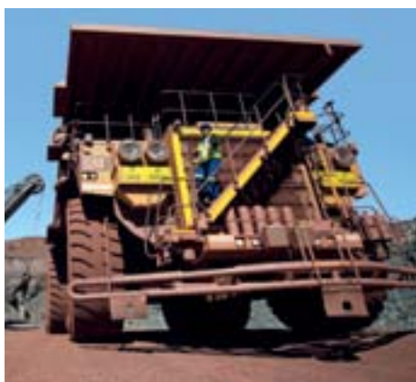
Driver/operator Deoni Adams about to continue her shift on a 280 tonne haul truck at Kumba's Sishen iron ore mine.
