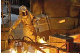
Collahuasi, Chile An operator working at the casting wheel, where molten copper is poured into moulds to form copper cathodes.
