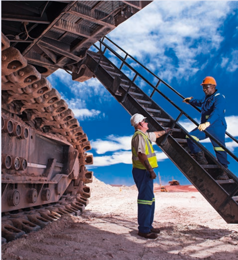
Image Mining safety officer Kobus Ellis and shovel operator Pitrus Skhungweni at Sishen mine. Next to them is a giant shovel, capable of delivering a payload of 108 tonnes in one scoop, which is being used to remove the calcrete overburden in the South Western portion of the pit.
