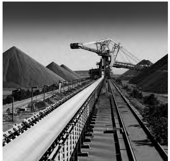
At Sishen, ore stockpiles are controlled by four stacker/reclaimers. Mining operations have been substantially reconfigured to reduce waste and to make the overall operation more resilient to future deteriorations in the iron ore price.
