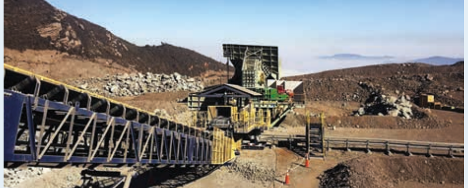
▲ A bulk ore sorting (BOS) machine operating in the open pit at Copper's El Soldado mine in Chile.
