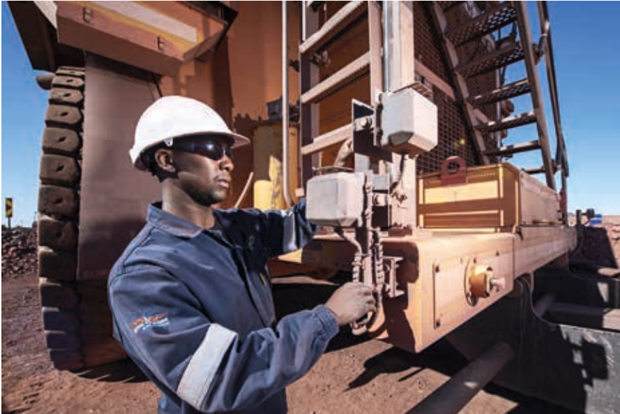
Fitment technician George Phirimi inspects the radar sensors, which are fitted front and rear, and cameras for the auto-braking system on a Komatsu 730 haul truck.
