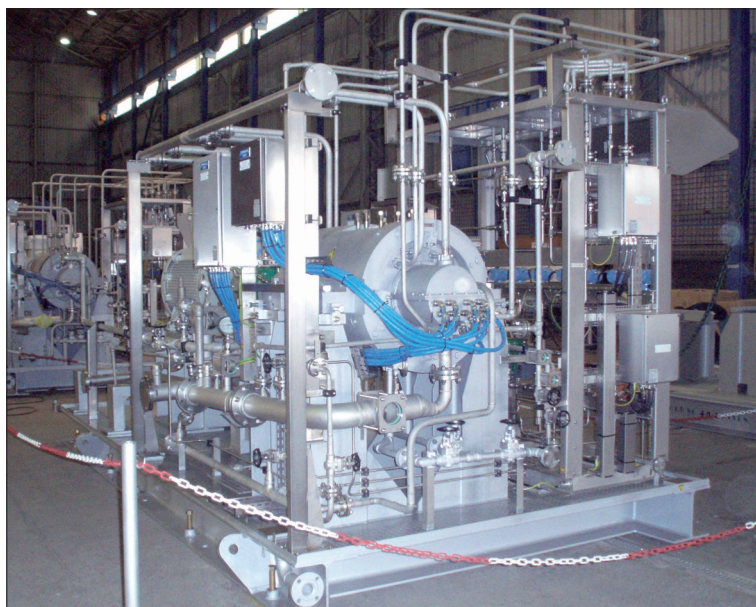
Image 4 (a) & (b) – Subba & Luhais Gas Compressors Ready for Shipment
