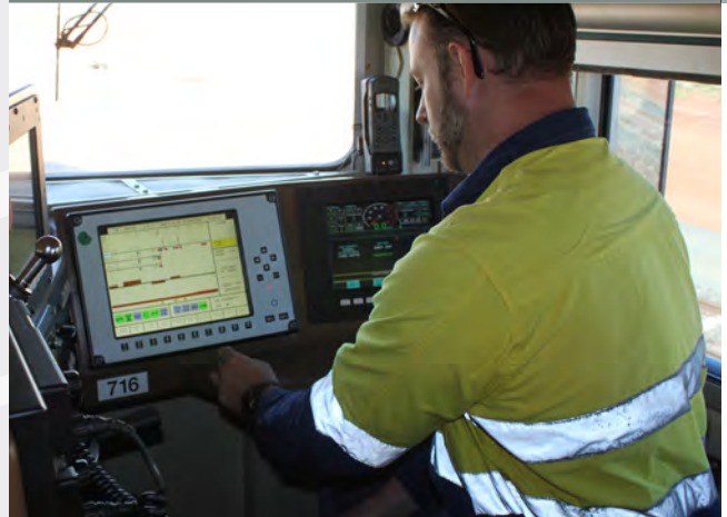
Incremental Train Control System
