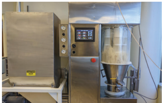
Granulation machine used to create a dry formulation for PREtec products.
