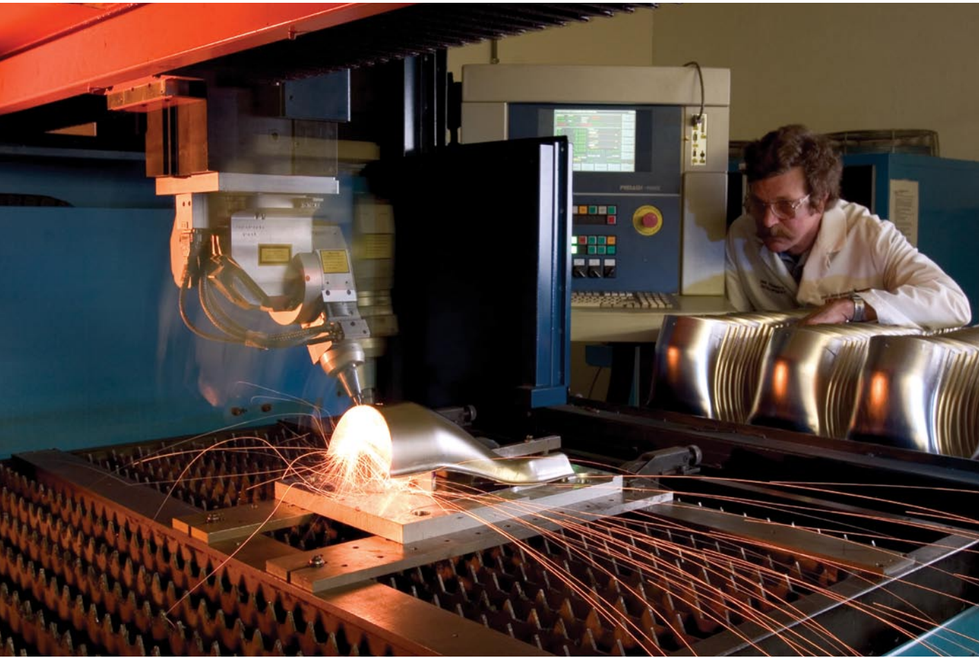
Above, a Flight Support Group manufacturing specialist monitors a Laser Cutting Machine System in the manufacture of aircraft parts.
