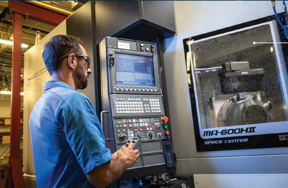
LEFT, A TEAM MEMBER IS PROGRAMMING A 5-AXIS CNC MACHINING CENTER AS IT MACHINES A CRITICAL ENGINE PART.
