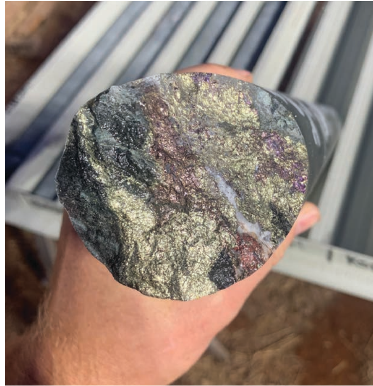
Cross section of mineralised core from diamond hole KSDD007 drilled at Boda, showing 2cm-thick bornite-chalcopyrite-quartz vein at 385m downhole.
