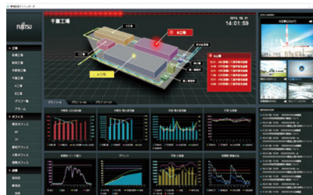
The "Environmental Management Dashboard" aggregates data on power usage volumes in real time and enables improvements in operational efficiency and reductions in CO 2 .
