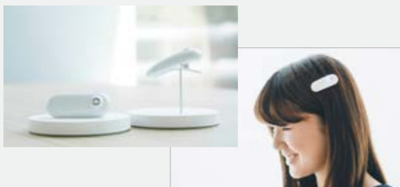
Ontenna, a groundbreaking device that uses haptic feedback to help the deaf interpret the world of sound around them
