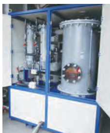
The waste liquid distillation concentrator deployed to Amatsuji Steel Ball Mfg. Co., Ltd. (Shiga plant)
