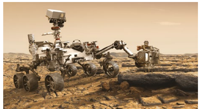
Cobham Advanced Electronic Systems: Cobham provides critical actuators on a number of space exploration vehicles, including the NASA Mars 2020 programme. These are used to drive the wheels, operate the steering and deploy the sensing mast among other critical applications. Credit: NASA
