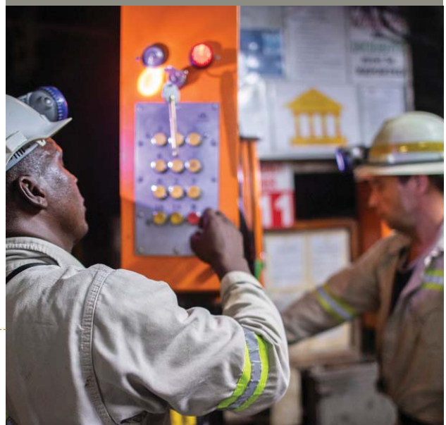
Barberton Mines – Fairview Mine 42 Level onsetter station >
