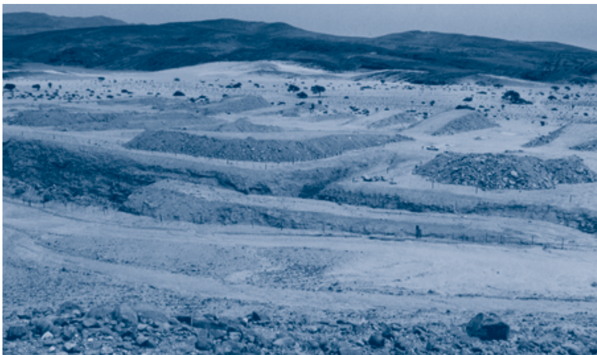
Test mining trench and pit (Gencor 1978). In background 21 dumps of graded ore for various lithological types.
