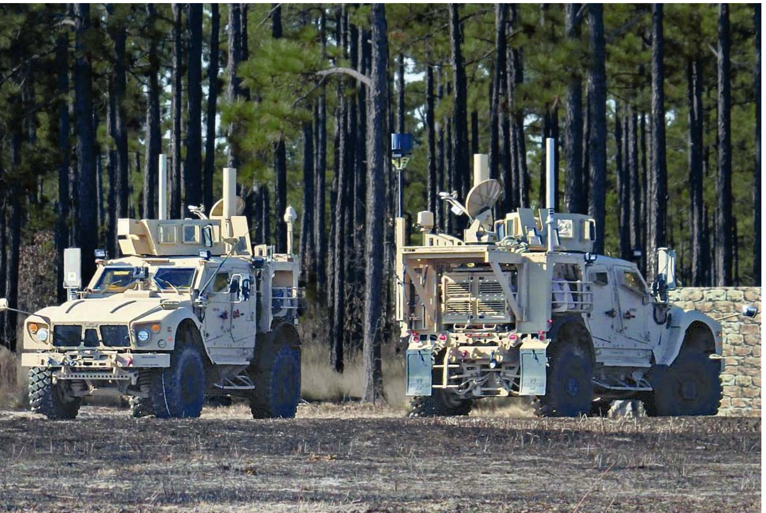
Vehicles equipped with the Prophet signals intelligence and electronic warfare suite produced by GD Mission Systems
