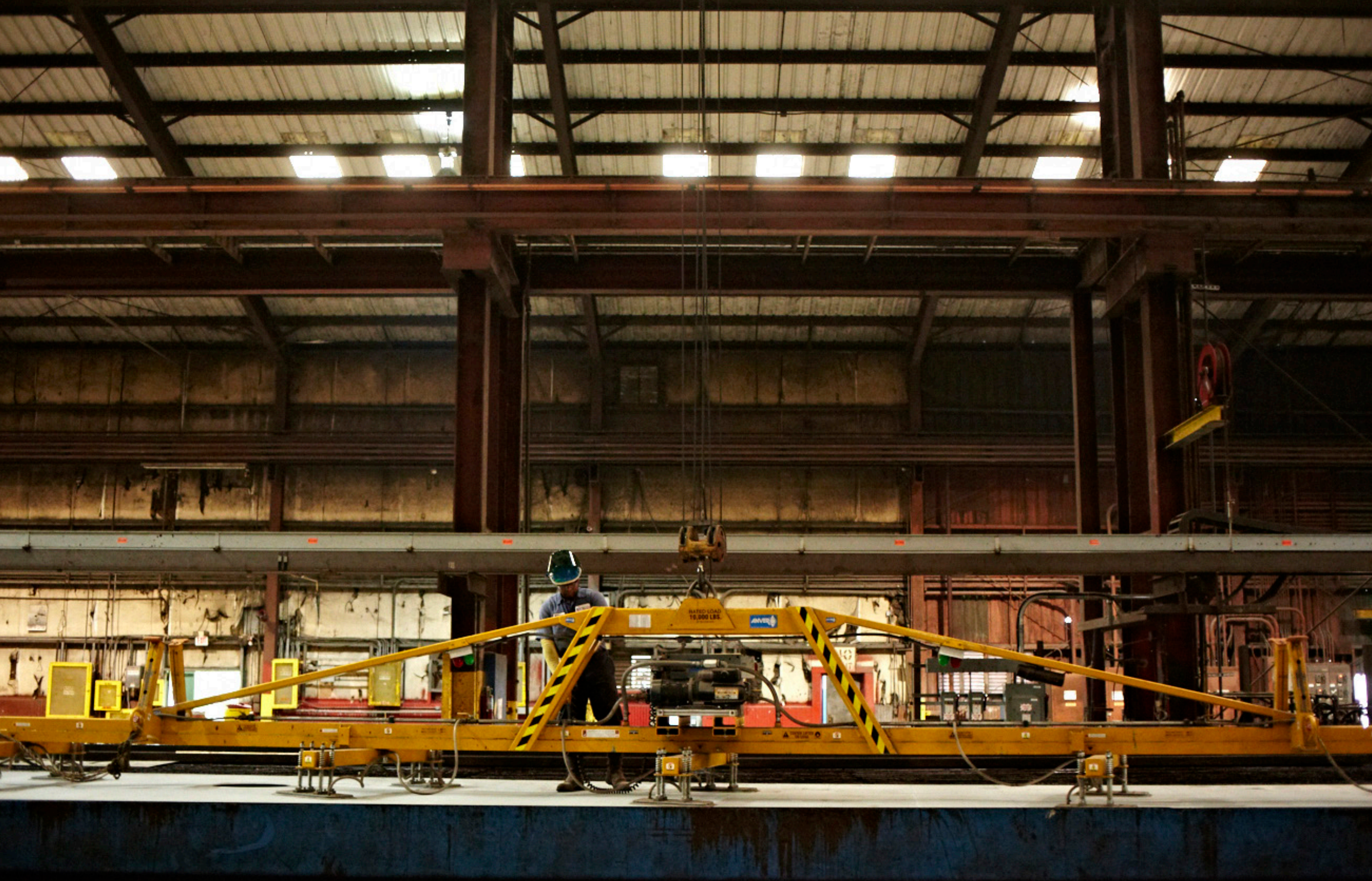
Antonio Banks of Metals USA unloading a finished cut part off the plasma table using a vacuum lift.
