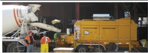
Capable of handling high psi and long distance pumping up to 1,000 feet vertically or 4,000 feet horizontally
