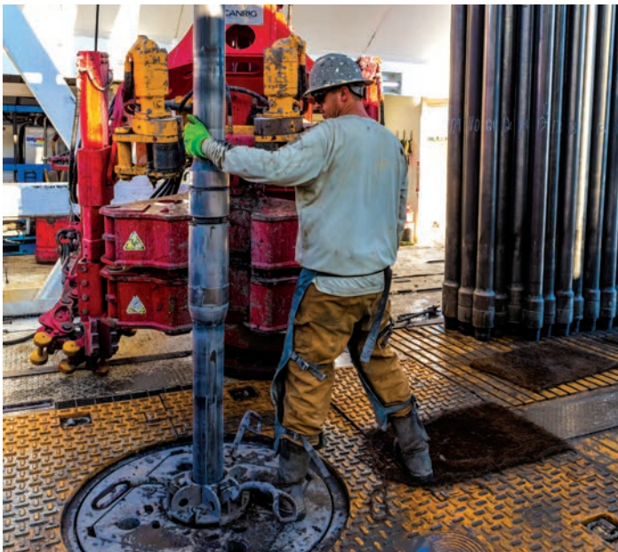
ABOVE: Worker on a drilling rig stacks pipe while drilling a Redtail well.
