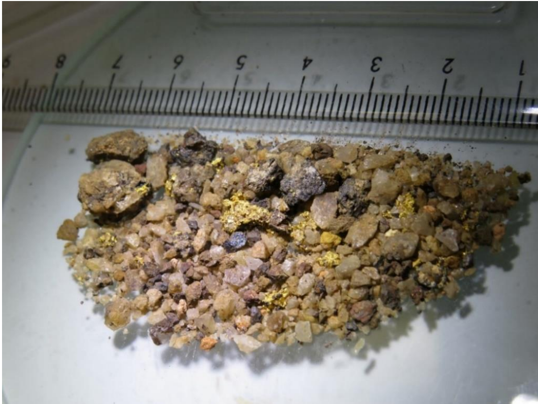
Figure 6. Visible gold within ferruginised quartz breccia (OGGRC266: 9-10m 794.2g/t Au)
