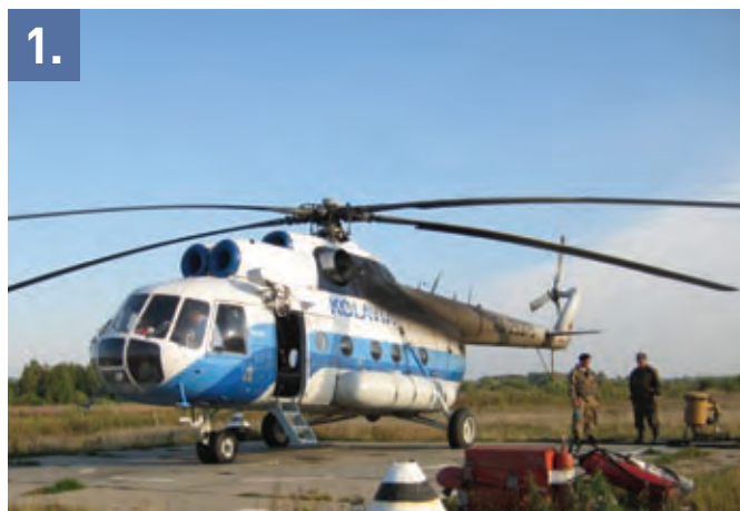
1. MI 8 helicopter used for crew change and supplies transport.
