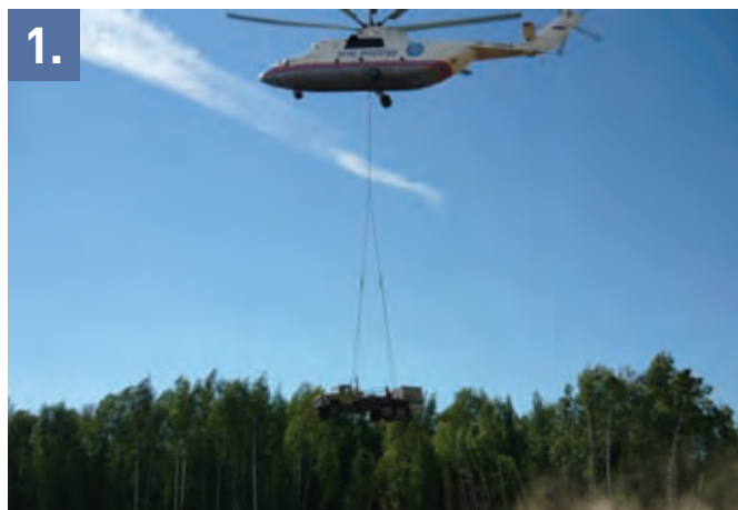
1. MI 26 helicopter transporting workover equipment to Lineynoye No.1 site.
