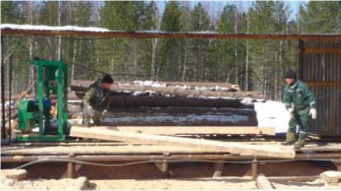
Sawmill in operation at Lineynoye oil field preparing timber for use in construction of new buildings.
