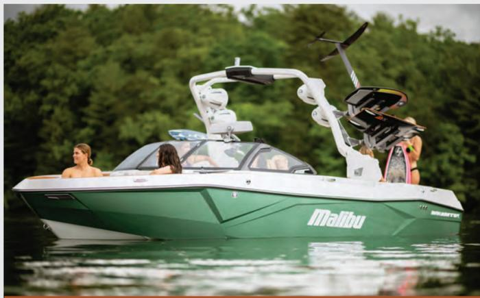
The electric G10+ TOWER™ folds down by simply turning a dial, allowing you to raise or lower your tower in a matter of seconds with just one hand.
