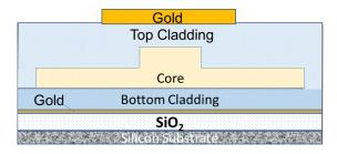
A ridge waveguide modulator is a type of modulator where the waveguide is fabricated within a layer of our electro-optic polymer system. Various cladding materials and electrodes are layered over the core polymer. The polymer materials are then part of an integrated photonics platform that can house other photonic devices, such as lasers, waveguides etc.
