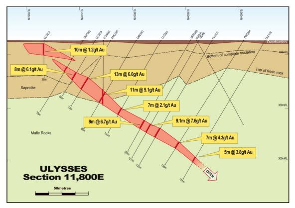
Figure 4 Ulysses Deposit Section 11,800E
