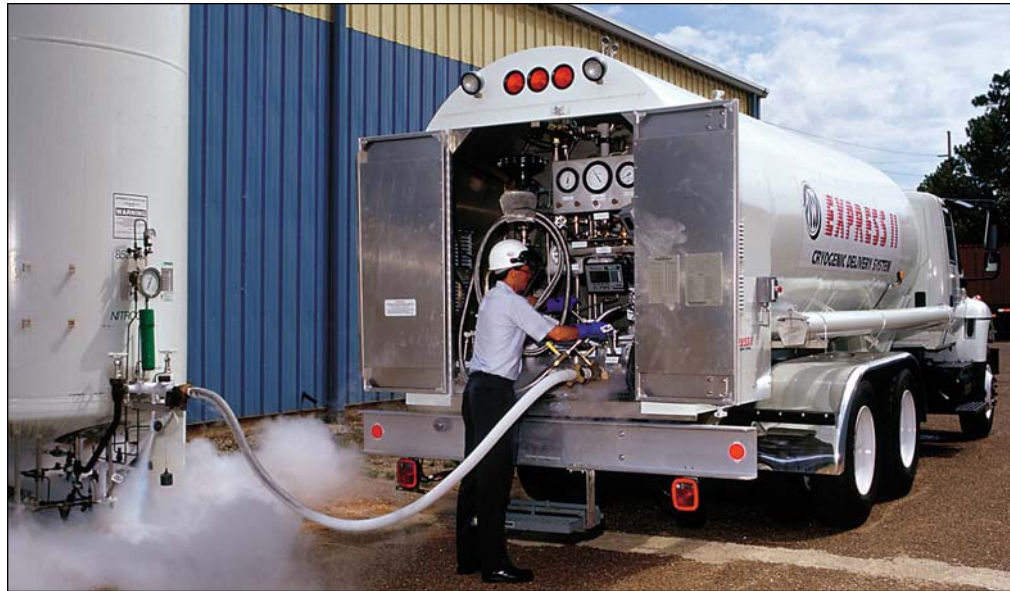
Taylor-Wharton's Express II cryogenic gas delivery system incorporates a unique "dual-hose" system that allows large bulk storage tanks as well as smaller liquid cylinders to be filled from the same mobile delivery truck. The Express II offers gas distributors the largest payloads available and is compatible with all cryogenic fill systems.
