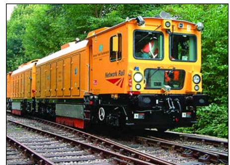
The U.K. has become a major international customer for Harsco's railway track maintenance services and equipment. This rail grinder for Network Rail is one of several units that Harsco will operate and maintain.
