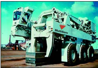
MultiServ's efficient on-site management of semi-finished materials is of critical importance to steelmaking operations. This specialized slab carrier can transport 100 tons of steel slabs.
