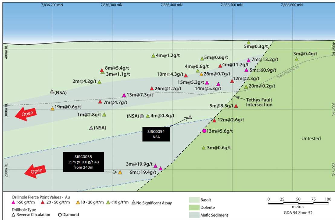
Figure 2 – Seuss North-South long section (ASX: 20 December 2018)
