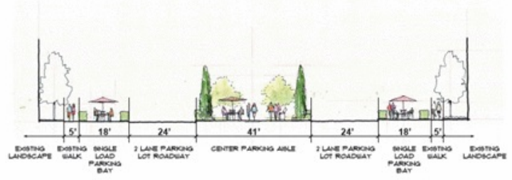
SECTION B SCALE 1/8"=1'-0"
