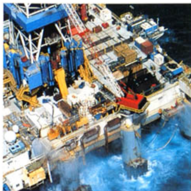
Timor Gap, Offshore Australia. The Atwood-Eagle, a semi-submersible rig drilling the successful Undan-1 well in ZOCA 91-12 during 1995.
