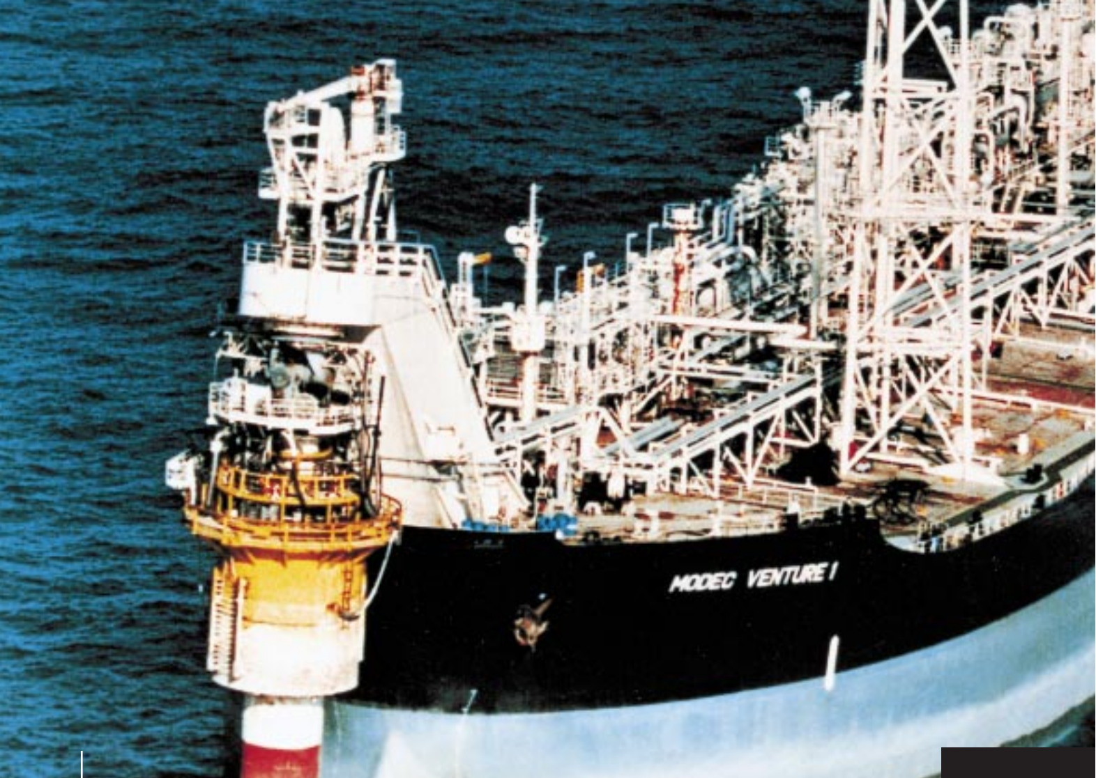
Modec Venture 1 floating production, storage and offloading facility (Elang/Kakatua/Kakatua North - Timor Gap)
