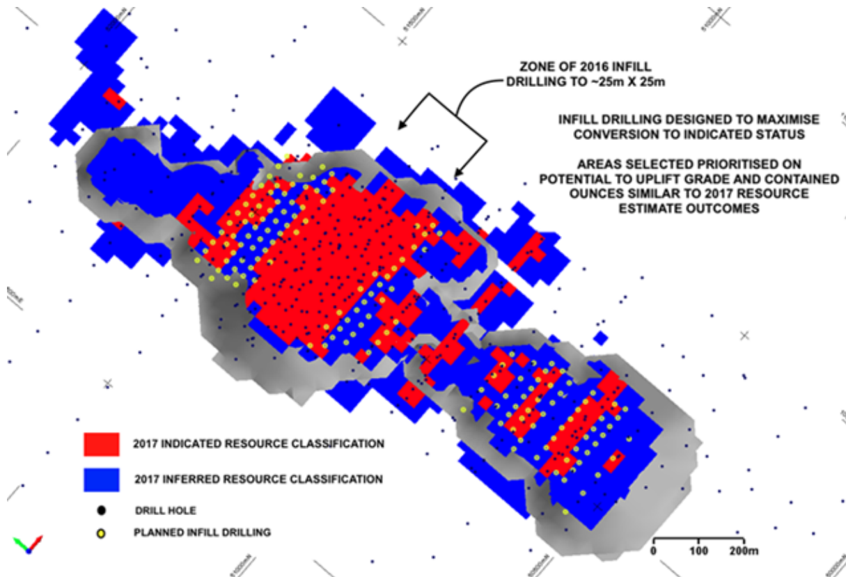
Figure 1: Paris Silver Project – Indicated Resource (red) and Inferred Resource (blue) – shown in plan within conceptual pit outline (grey), with planned drilling (yellow dots) and historical drilling (black dots)
