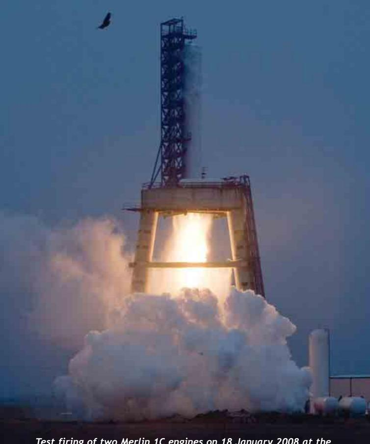
Test firing of two Merlin 1C engines on 18 January 2008 at the SpaceX test facility in McGregor Texas. Powered by liquid oxygen and rocket grade kerosene, the pair of Merlins produced over 181,000 pounds of thrust during the test. A total of nine Merlin 1C engines will power the Falcon 9 rocket.
