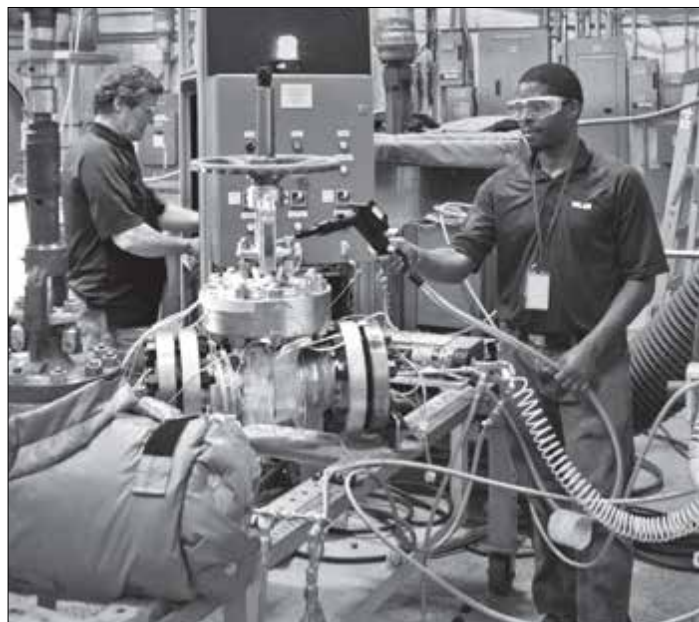
Fugitive emissions testing of a 4" (100 mm) Class 600 cast steel gate valve.
