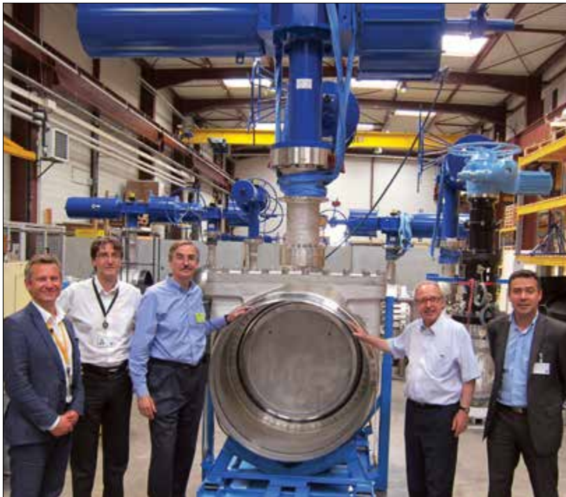
Members of the Velan France executive team with Tom Velan standing in the Velan S.A.S. manufacturing plant in Lyon, France, next to a 36" (900 mm) top-entry cryogenic butterfly valve ready for shipping to an LNG facility.
