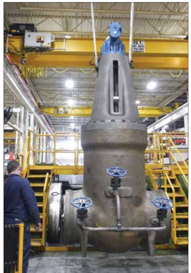
Hydrotesting of large high-pressure valves in one of Velan's Montreal plants. This is one of four 36" Class 900 parallel slide valves for SAGD service in Western Canada.
