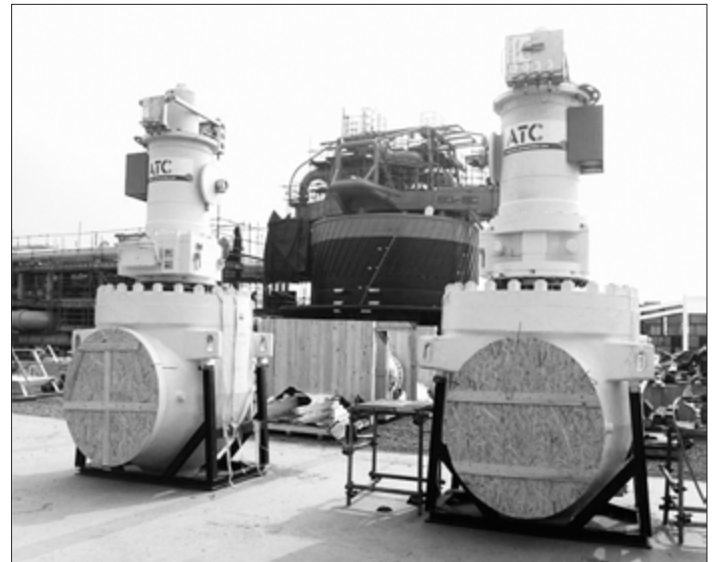
Two 48" Class 300 top-entry subsea ball valves manufactured in Italy by Velan ABV for a refinery and petrochemical plant in Vietnam. The valves weighed 40 tons each.
