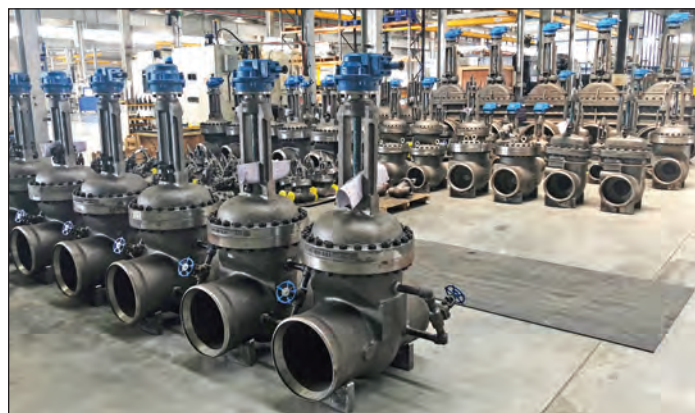
Cast steel valves for NTPC Telangana supercritical power plant manufactured and ready for shipment from our Velan Valves India location.
