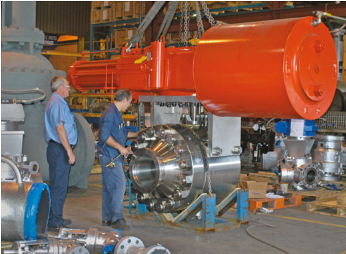
Velan R-series metal-seated ball valve, designed for a high pressure and corrosive hydrogen and sulphur-rich innovative industrial process in the petrochemical industry.
