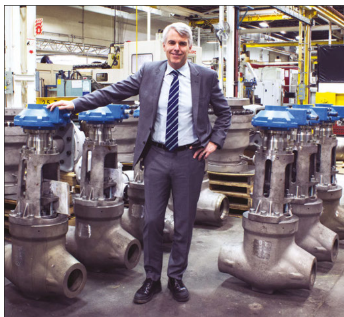
Yves Leduc, Velan Inc's President and Chief Executive Officer next to a group of 8" gear operated nuclear globe valves, manufactured in Canada.
