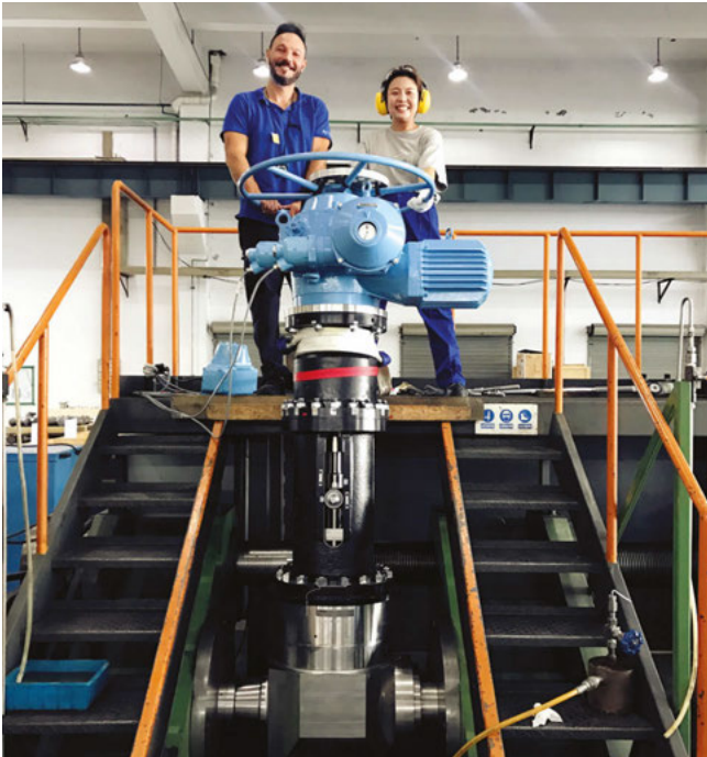
That's teamwork! Manufactured by Velan S.A.S. in France, this valve was sent to Velan China's Suzhou plant for hydrotesting before reaching its destination in one of China's nuclear power plants.
