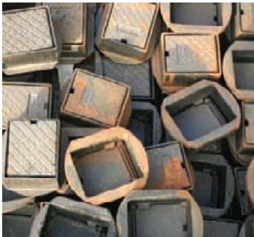
Stop tap boxes, which are supplied to local authorities throughout the country
