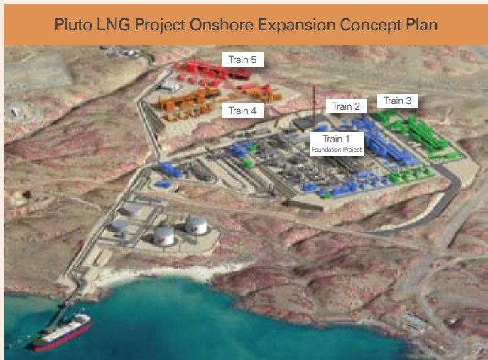
Pluto LNG Park expansion concept plan showing possible location of up to four additional LNG trains
