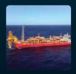
Offshore, crude oil from Enfield is produced into the *Nganhurra* floating production storage and offloading vessel before shipment to refiners.
