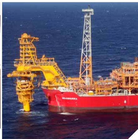
The Nganhurra floating production storage offloading (FPSO) vessel is one of four FPSO's in Woodside's fleet. Oil is produced through five subsea wells connected to the vessel.
