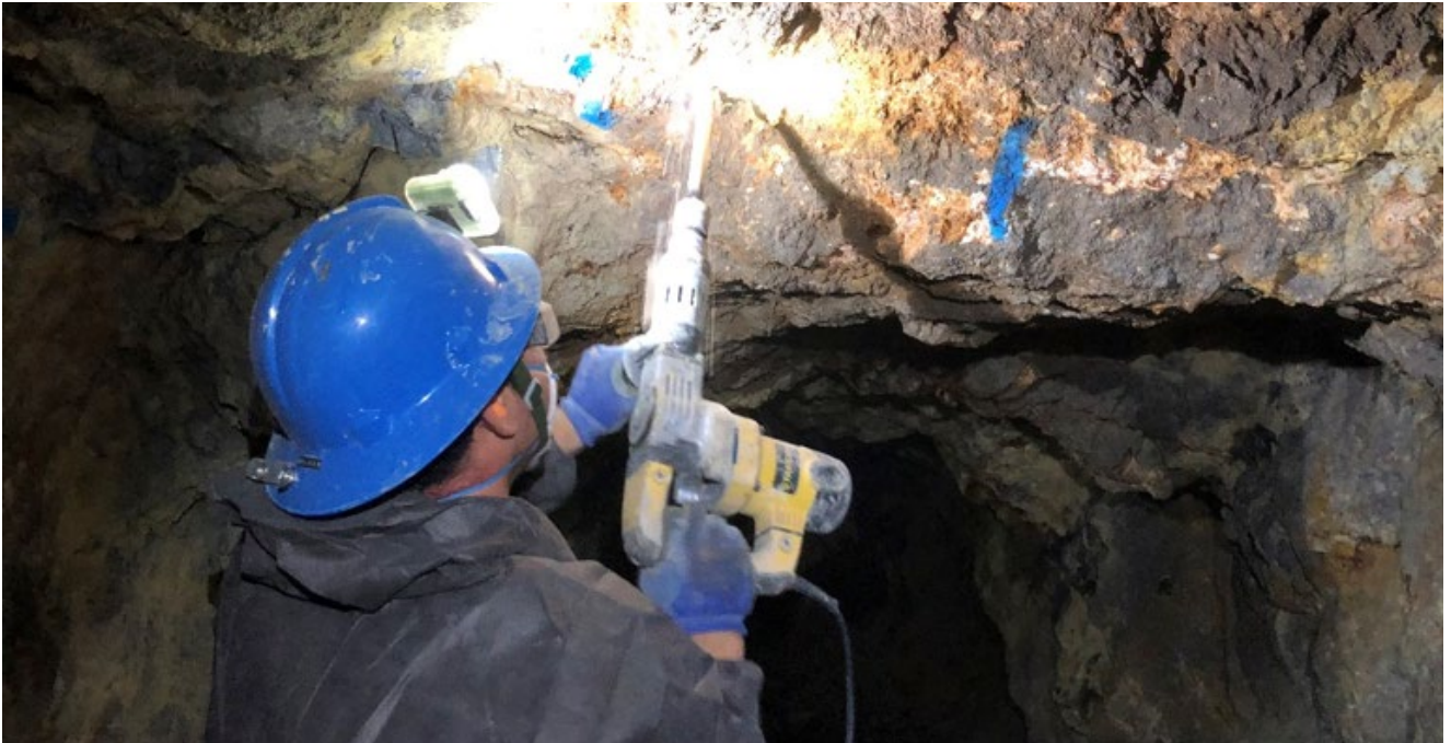
Channel sampling of the Shin Adit, Deokon Gold-Silver Project, South Korea
