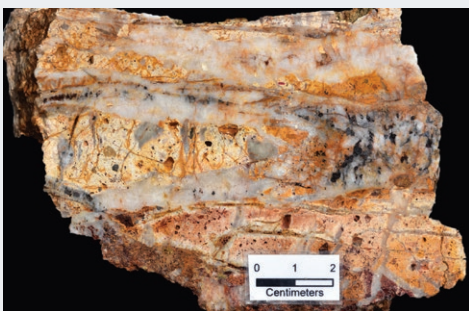
Top: Slab photos of samples KRS205352 78.6g/t Au and 13,000g/t Ag (upper sample) and KRS206389 6.8g/t Au and 1010g/t Ag (lower sample) both float samples from the Bonanza Zone with visible native silver and electrum in hand specimen. Bottom: Float sample KRS206272, 35.1g/t Au and 3270g/t Ag . Golden Surprise, Bonanza Zone .
