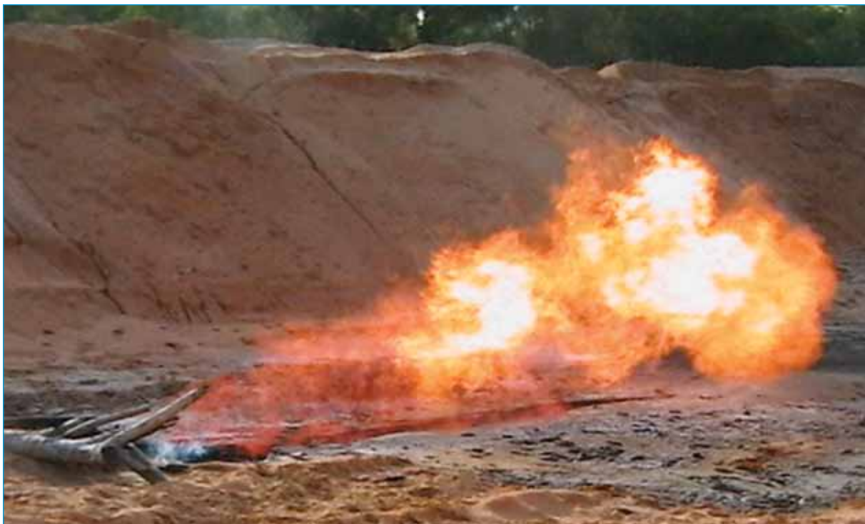
Gas flowing during production testing at Advent Energy's Waggon Creek-1 well in EP386.
