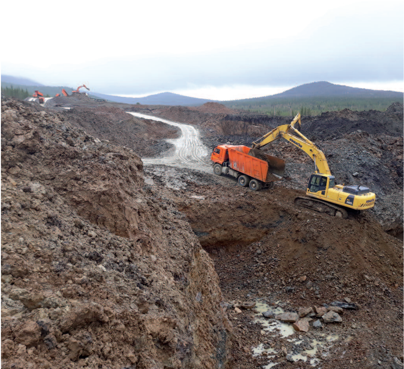
Above, two Komatsu excavators loading a fleet of four trucks at Malaya Sosnovka in May 2018. At the washplant, visible in the background, a third excavator loads material into the trommel.
