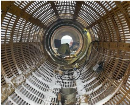
Figure 4: A welder undertaking maintenance on a trommel and scrubber at site in 2021. This mechanism rotates at speed and with the addition of water, delivered at pressure, disintegrates gravel and river sediments. Further beneficiation steps are mechanical, and gravity assisted with no chemicals used in the entire process which results in a 'black sand' PGM, Chrome and Iron concentrate which is shipped to a refinery in Ekaterinburg.
